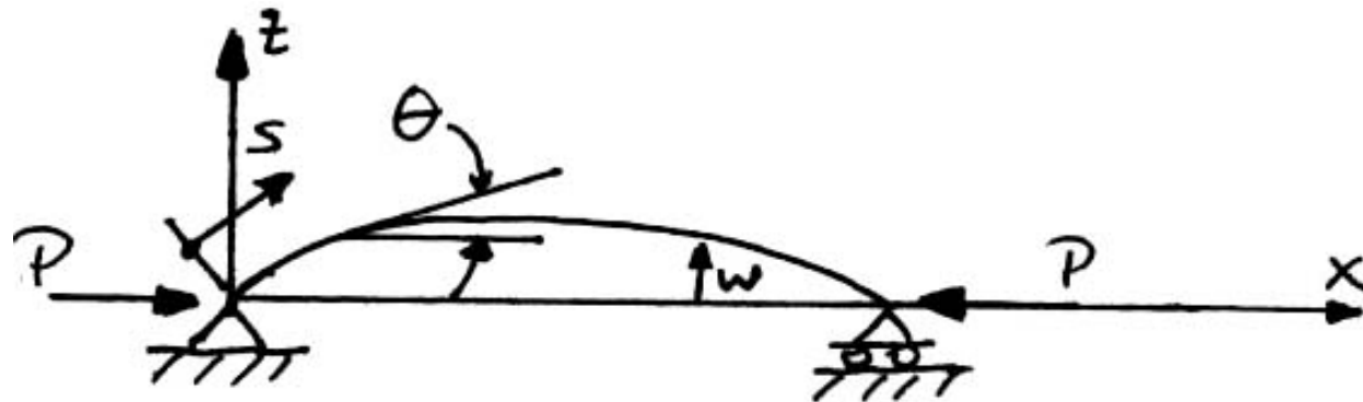
Figure 18.13 Representation of post-buckling of a beam-column
