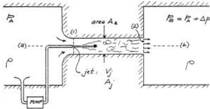
The device connected between compartments A and B is a simplified version of a jet pump. A jet (or ejector) pump is a device which uses a small, very high-speed jet with relatively low volume flow rate to move fluid at much larger volume flow rates against a pressure differential  $\Delta p$ , as shown in the figure.
