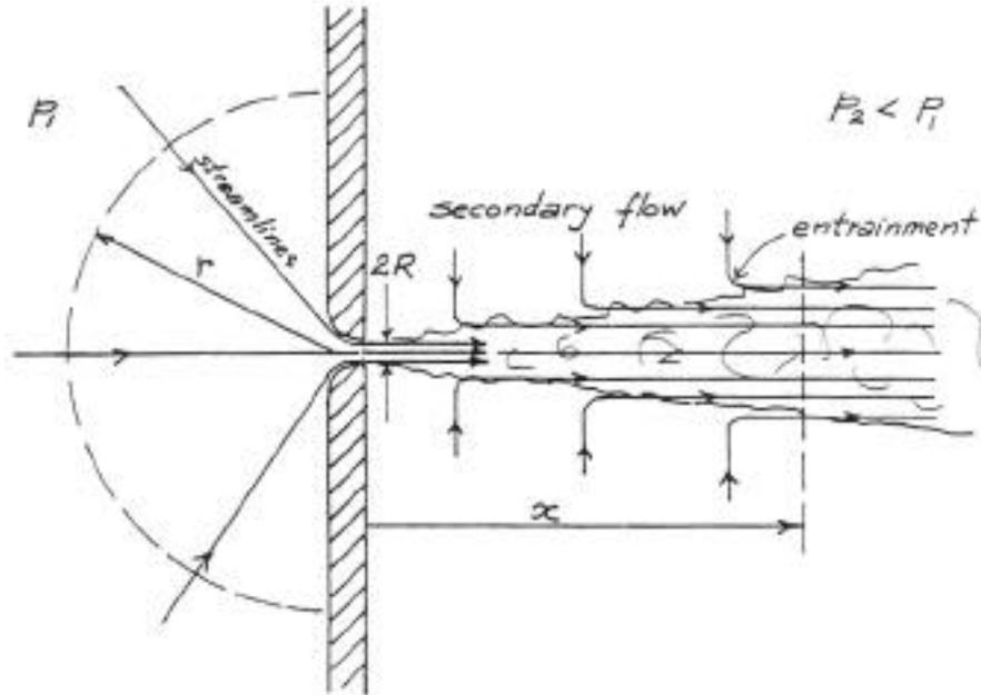
A wall in which there is a small nozzle, or hole, of radius  $R$ , separates two large compartments. The pressure  $p_1$  in the left-hand compartment far from the nozzle is greater than the pressure  $p_2$  in the right-hand compartment, and a steady volume flow  $Q$  takes place from 1 to 2.
