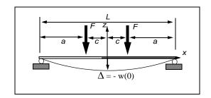
To deduce an expression fro the midspan displacement of the beam shown at the left - load P is concentrated at mid-span, we set a = L/2, and F = P/2. (Think of moving the two loads, each of magnitude *F*, in toward the midspan, shrinking *c* to zero).
