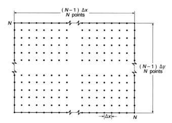
Figure 1.1: Square, homogeneous grid used for discretizing the Laplacian, thus reducing the {grid1.tif} partial differential equation to a set of linear simultaneous equations.
