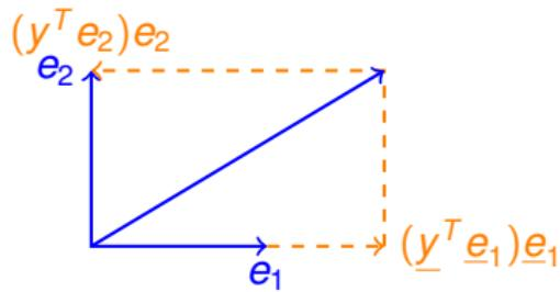
$$\pi_d(y_n) = (\underline{y}^T \underline{e}_1) \underline{e}_1 + (\underline{y}^T \underline{e}_1) \underline{e}_1$$
