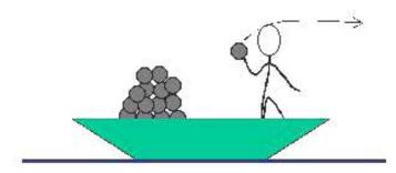
R = throwing rate (rocks/s) m<sub>b</sub> = mass of boat and everything in it (kg) m<sub>r</sub> = mass of one rock (kg) u<sub>r</sub> = velocity of rock relative to boat (m/s) u<sub>b</sub> = velocity of boat (m/s)
