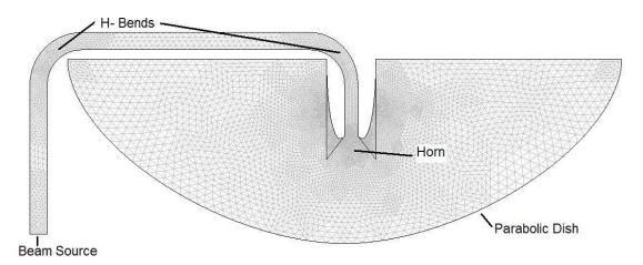
Figure 1. Microwave circuit CAD model and 2D FEM mesh.
