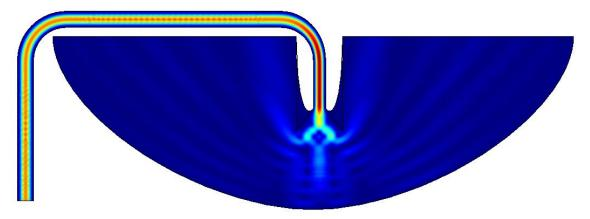
Figure 2. Power flux output plot. Dark blue corresponds to 130 W/m<sup>2</sup>. 127 W/m<sup>2</sup> is required to furnish 400W to a 2m diameter rectenna.
