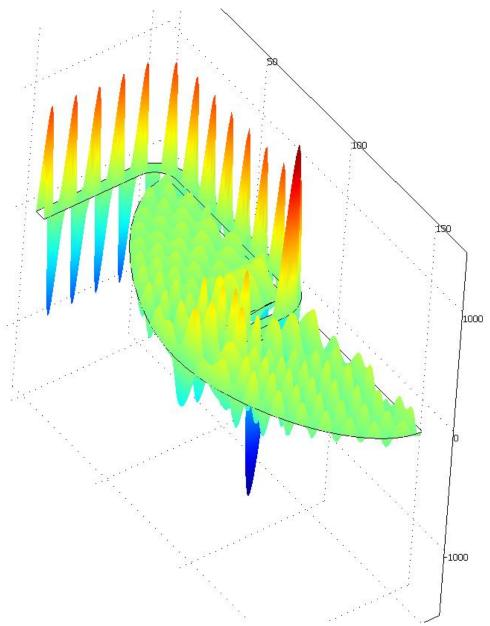
Figure 3. z-component of the Electric field of the microwaves inside the waveguides and antennae. The extremum peaks (red and blue) are 1300V/m and -1400V/m respectively.
