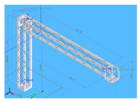
Figure 1. Stand CAD model and 2D FEM mesh.
