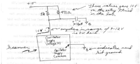
Note that I've not shown the cable connections. You can work these out.
