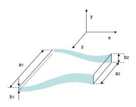
A steady, inviscid, incompressible flow experiences a change of cross sections between stations (1) and (2), as shown. At station (1), the velocity distribution is
