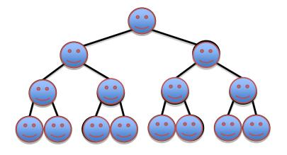
Observe however that Max\_Heapify takes O(1) for time for nodes that are one level above the leaves, and in general, O(l) for the nodes that are *l* levels above the leaves. We have n/4 nodes with level 1, n/8 with level 2, and so on till we have one root node that is lg n levels above the leaves.
