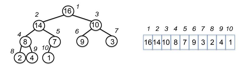
No pointers required! Height of a binary heap is O(lg n)
