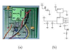
Figure 4: Picture and schematic of the sensor equipped with an accelerometer, ADC and LEDs.
