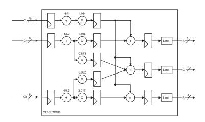
Figure 8: Hardware Implementation for the Conversion of the YCrCb to RGB.
