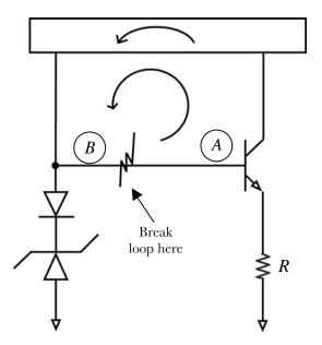
After loop is broken, raising node (A) causes (B) to rise! We don't get into trouble because the gain around the loop is small (<1).
