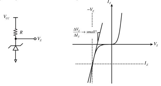
A good Zener diode will have a small incremental resistance,  $r_z$ . If we write out the response of the output voltage to changes in the supply, we get:
