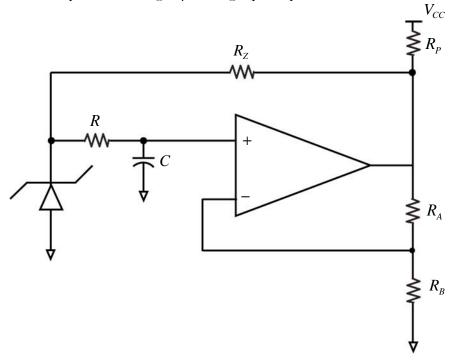
$R_{p}$  can be chosen to provide much of the Zener current. In addition, it helps with <u>startup</u> for this circuit.
