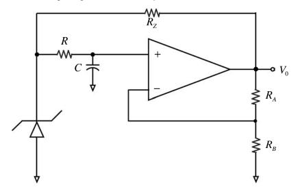
Notice that the op-amp is just connected as a non-inverting amplifier of gain k. For purposes of the DC bias calculation, notice that R and C have no impact.
