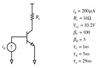
We ask, how long does it take to get out of cutoff? In order to get out of cutoff,  $V_{BE}$  must equal 600mV. In order to get  $V_{BE}$  to 600mV, we must charge  $Q_{VE}$  and  $Q_{VC}$  appropriately. The total amount of charge needed is
