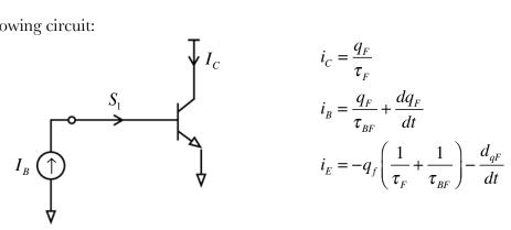
At time t=0, we open switch  $S_1$ . Derive and sketch  $I_C$  as a function of time.
