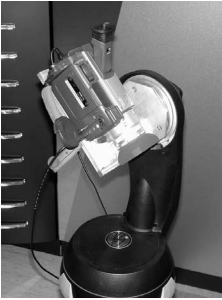
Figure 2: Digital video camera mounted on fork arm.
