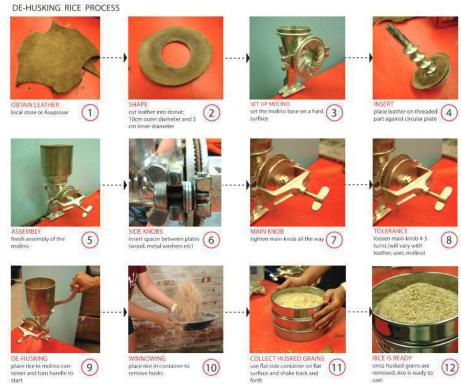
Figure 5. The 12 step de-husking process proposed
