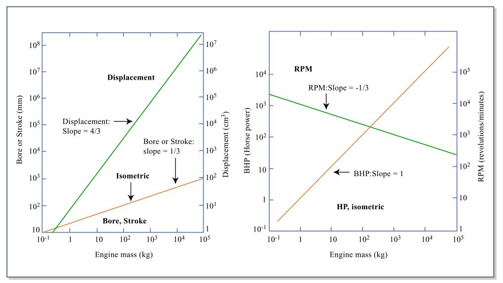
Stroke\* $\omega$  = peak piston velocity = const Peak specific strain energy = const Internal Structure 4/6/06 © Daniel E Whitney Figure by MIT OCW. After McMahon and Bonner.
