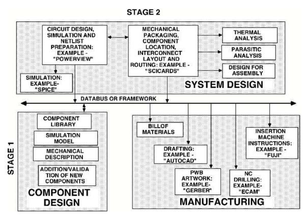
Figure 1. Sketch of VLSI System Design and Manufacturing
