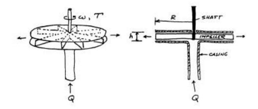
The sketch shows an impeller with radial vanes in a flat-sided casing of radius R and height h. The impeller is mounted on bearings and is free to rotate without friction, but the casing is held stationary. Fluid of density  $\rho$  enters the impeller via a pipe which has a radius small compared with R. The velocity in the pipe is purely axial, and the volume flow rate is steady at a value Q.
