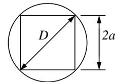
The torsional stiffness of the solid circular shaft is  $\pi R^4/2$ . That for the square shaft is obtained from the textbook, page 232. There we find  $M_t = K_t \cdot \phi/L$  where  $K_t = G \cdot k_1 \cdot (2a)^3 (2b)$ . In terms of the radius of the circle, putting  $a$  (and  $b$ ) in terms of the radius  $R$ , gives
