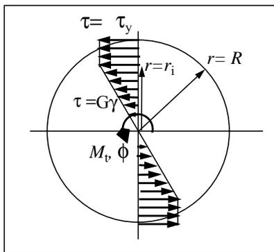
Consider the shear stress distribution at some instance *beyond* the onset of yield. Onset of yield will occur when the shear stress at the outer radius of the shaft,  $r = R$ , attains the value  $\tau_y$ . With some additional loading, some additional torque applied, the shear stress distribution over the radius might appear as at the left.
