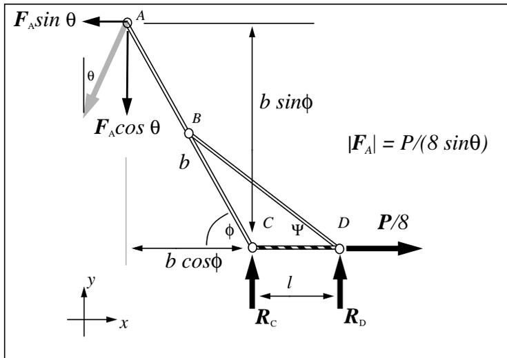
**The equilibrium equations** whose solution will give the reaction forces at C and D. Note that the resultant of the two horizontal components is zero. So we need only consider the resultant moment and the resultant of the vertical, y, components. We reference moments to the point C below.
