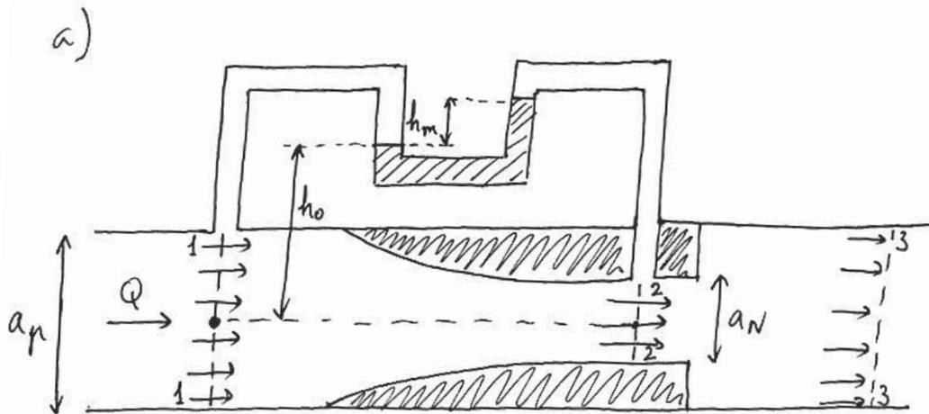
At 1-1 and 2-2 we have well-behaved flow and pressure is hydrostatic. With this, from the manometer reading, we can obtain the pressure difference between 1 and 2:
