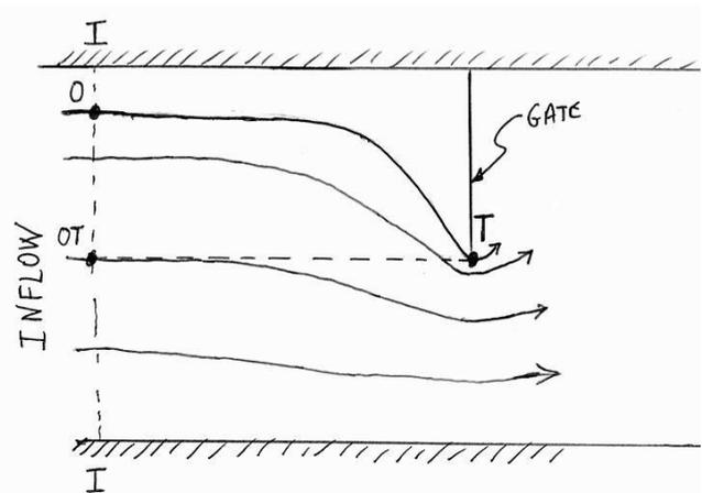
$p + \rho gh$  (because flow is well behaved in I-I and pressure varies hydrostatically), and also the same value of the velocity (because flow is uniform at the inflow). However, this is just luck, and in general you can only apply Bernoulli between two points on the same streamline.
