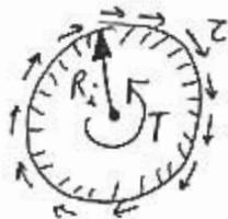
$$T = \underbrace{|\tau| \cdot 2\pi R_i l}_{\text{force}} \cdot \underbrace{R_i}_{\text{arm}} = \frac{2\pi R_i^3 l \omega}{R_o - R_i} \mu$$
