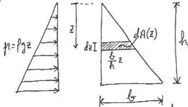
$$\begin{aligned} \text{PRESSURE FORCE} = \underline{F_P} &= \int_0^h p(z) dA(z) = \int_0^h \rho g z \frac{b}{h} z dz = \\ &= \frac{\rho g b}{h} \int_0^h z^2 dz = \frac{\rho g b}{h} \frac{h^3}{3} = \underline{\underline{\frac{1}{3} \rho g b h^2}} \end{aligned}$$
