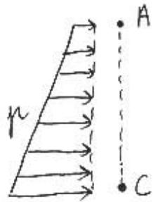
$$\begin{aligned} \underline{p_{A, \text{abs}}} &= p_{C, \text{abs}} - \rho g h = p_{\text{ATM, abs}} - \rho g h = \\ &= 101300 - 1000 \cdot 9.8 \cdot 10 = \underline{\underline{3300 \text{ Pa}}} \end{aligned}$$
