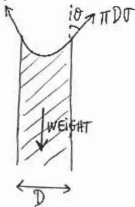
$$\underbrace{\rho g \frac{\pi D^2}{4} h}_{\text{WEIGHT}} = \underbrace{\pi D \sigma \cos \theta}_{\text{SURF. TENSION}} \Rightarrow D = \frac{4 \sigma \cos \theta}{\rho g h}$$
