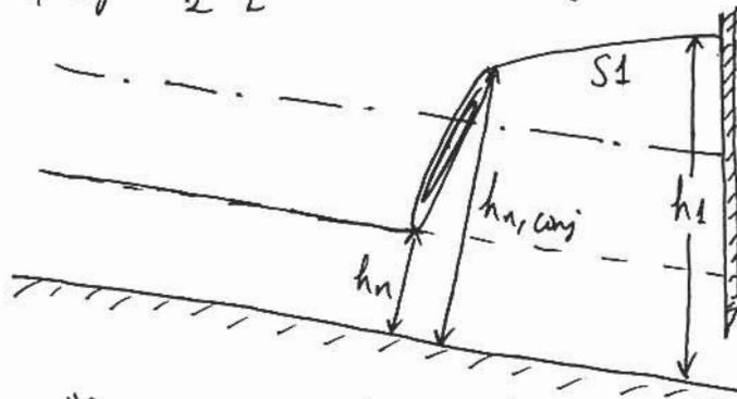
$$\begin{aligned} h_n &= 1.25 \text{ m} \\ h_{n, \text{conj}} &= 1.49 \text{ m} \\ h_1 &= 3.96 \text{ m} \end{aligned}$$
