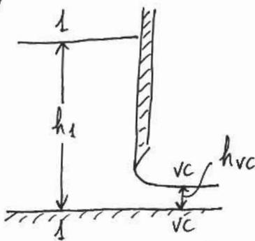
Depth at V.C.:  $h_{vc} = C_v \cdot h_s = 0.61 \text{ m}$ .
