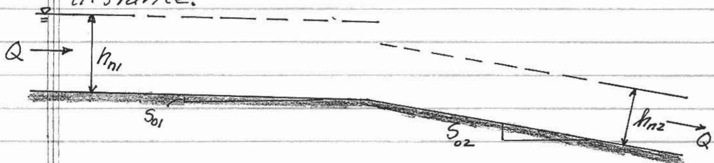
Far upstream and downstream of the change in bottom slope the flow must be uniform, since this is the only flow that can exist in an "infinitely long" channel. But if this were the case all the way to the sudden change in slope, then the mismatch in depths ( $h_{n1} \neq h_{n2}$ ) could only be handled by out "rapidly varying flow" tools if  $h_{n1}$  and  $h_{n2}$  were either ALTERNATE or CONJUGATE DEPTHS.
