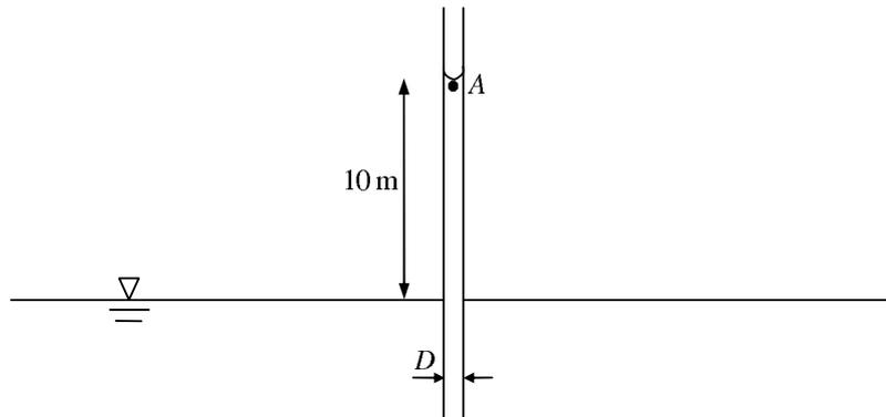
Figure 1: Capillary tube in Problem 2.
