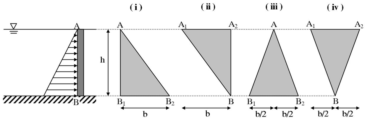
Figure 3: Submerged triangular plates in Problem 4.
