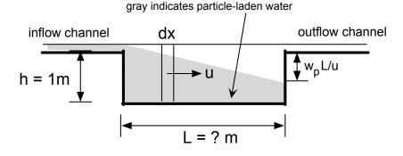
The above picture shows how the region of particle-laden water evolves across the pond. The picture suggests that if outflow is drawn from the surface, it will be free of particles, *i.e.* the effective removal can be 100%.
