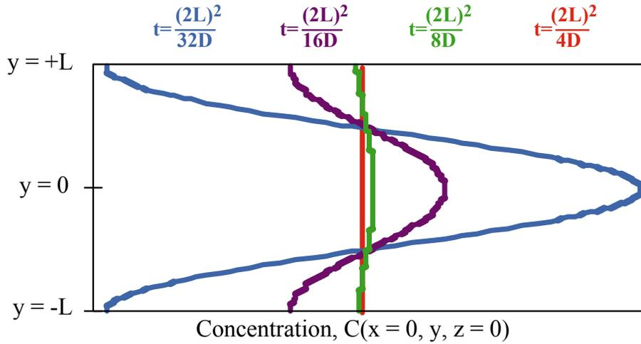
**Figure 5.** A slug of mass is released at  $(x, y, z, t)=0$  into a fluid domain that is unconstrained in the  $x$ - $z$  plane, but is constrained by parallel, no-flux boundaries at  $y = +L$  and  $-L$ . The profiles of concentration,  $C(x=0, y, z=0)$ , are plotted for several times after the release. The system is fully mixed (uniform) across the  $y$ -domain in a time  $t = (2L)^2/4D$ .
