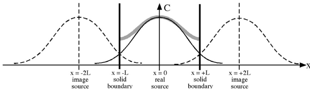
**Figure 3.** To satisfy the no-flux condition at both boundaries, two image sources (dashed) are added to the real source (black). For short time, the sum of these three sources (gray) is sufficient to satisfy  $\partial C / \partial x = 0$  at  $x = \pm L$ . However, at later time each image source will begin to lose mass across its opposite boundary, and the no-flux condition will no longer be satisfied. Ultimately, images will be needed at  $x = \pm 2nL$ , for all integer  $n$ .
