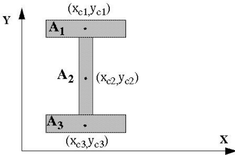
$$x_c = \frac{\sum_{\text{sections}} A_i \cdot x_{ci}}{\sum_{\text{sections}} A_i} \quad y_c = \frac{\sum_{\text{sections}} A_i \cdot y_{ci}}{\sum_{\text{sections}} A_i}$$
