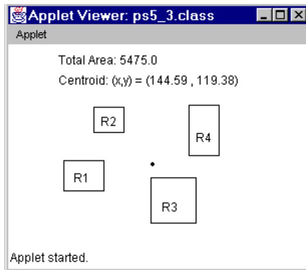
The centroid of a set of shapes is computed as the sum of the products of the area of each shape times its centroid coordinate ( $X_{ci}$  and  $Y_{ci}$ ) divided by the total area of the cross-section. For example, the centroid ( $X_c, Y_c$ ) of the following section is defined by the following formulas:
