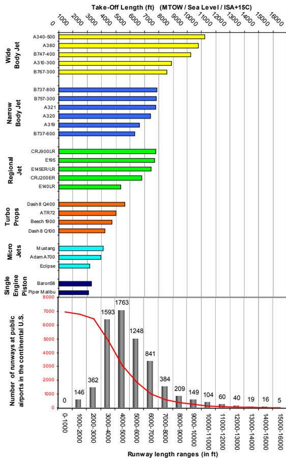
**Figure 2: Aircraft performance vs. airport capabilities in the United States [4] [5].**
