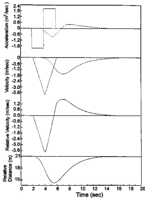
Note: Vehicle 2 follows Vehicle 1 (lead car) with a time lag  $T=1.5$  sec and a value of  $C=e^{-1}(\approx 0.368)$ , the limiting value for local stability. The initial velocity of each vehicle is  $u$
