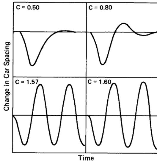
Note: Changes in car spacings from an original constant spacing between two cars for the noted values of C. The acceleration profile of the lead car is the same as that shown in Figure 4.2.
