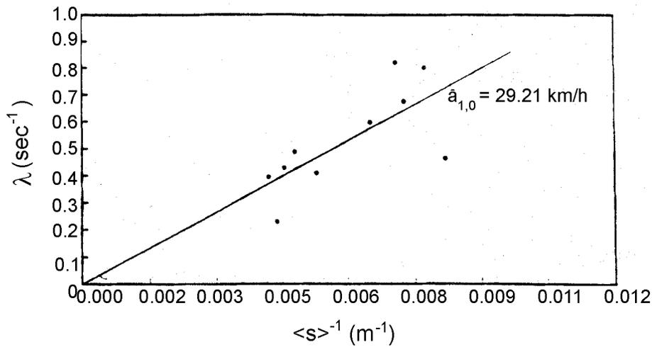
Note: The straight line is a "least-squares" fit through the origin. The slope, which is an estimate of  $a_{1,0}$  equals 29.21 km/h.
