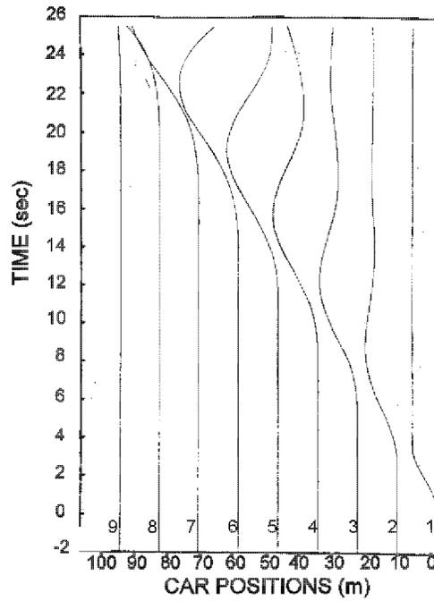
Note: Diagram illustrates the linear car following equation, eq. 4.23, where  $C=0.80$ .
