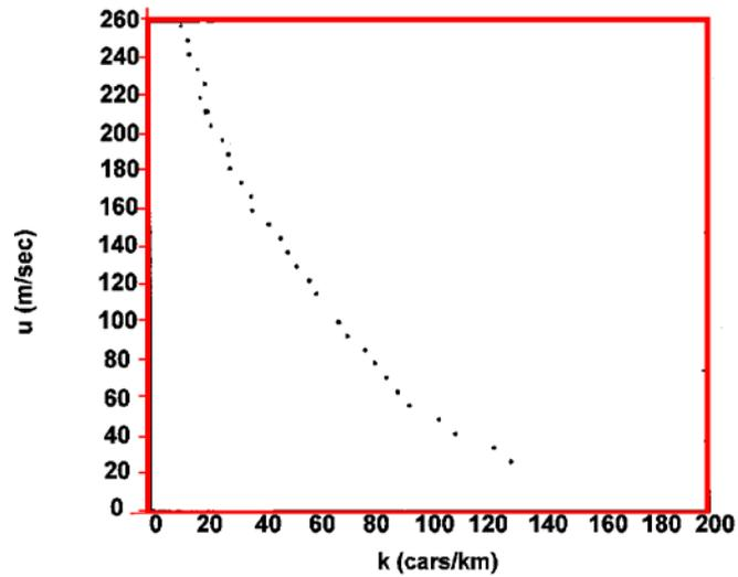
Note: Each data point represents a speed class of vehicles moving with the plotted speed  $\pm 1$  ft/sec (See Table 4.4).
