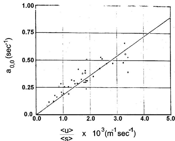
Note: The sensitivity coefficient versus the ratio of the average speed to the square of the average spacing for each bus following experiment. The least squares straight line is shown. The slope of this regression is an estimate of the speed-reciprocal spacing squared sensitivity coefficient. The solid dots and circles are data points for two different test runs.
