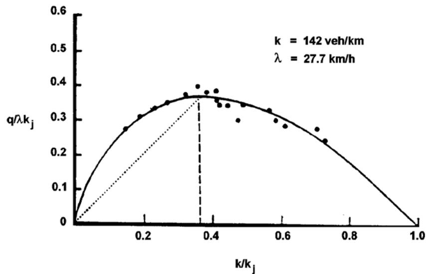
Note: The curve corresponds to Equation 4.40 where parameters are those from the "fit" obtained in Figure 4.11.
