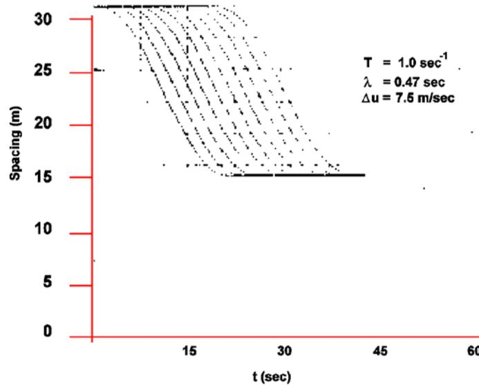
Note: A numerical solution to Equation 4.32 for the inter-vehicle spacings of an 11- vehicle platoon going from one steady-state to another ( $\lambda T = 0.47$ ). The lead vehicle's speed decreases by 7.5 meters per second.
