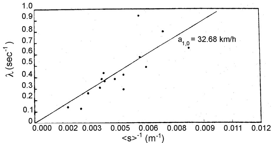
Note: The straight line is a "least-squares" fit through the origin. The slope, is an estimate of  $a_{1,0}$  equals 32.68 km/h.
