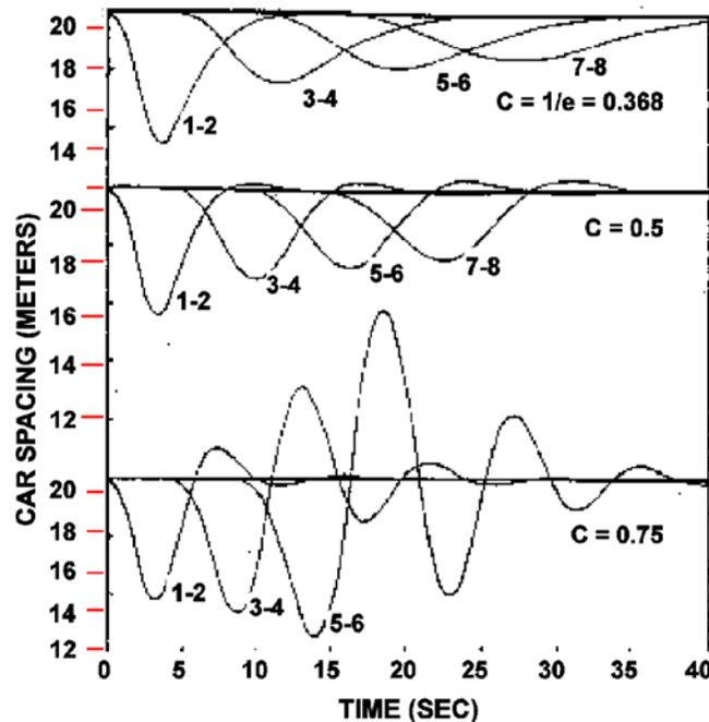
Note: Diagram uses Equation 4.23 for three values of  $C$ . The fluctuation in acceleration of the lead car, car number 1, is the same as that shown in Fig. 4.2. At  $t=0$  the cars are separated by a spacing of 21 meters.
