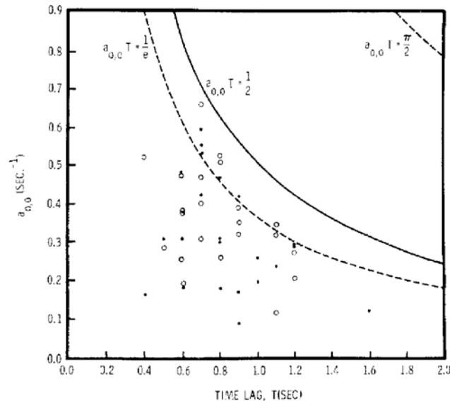
Note: For bus following experiments - Some drivers are represented by more than one test. The circles are test runs by drivers who also participated in the ten bus platoons experiments. The solid curve divides the graph into regions of asymptotic stability and instability. The dashed lines are boundaries for the regions of local stability and instability.
