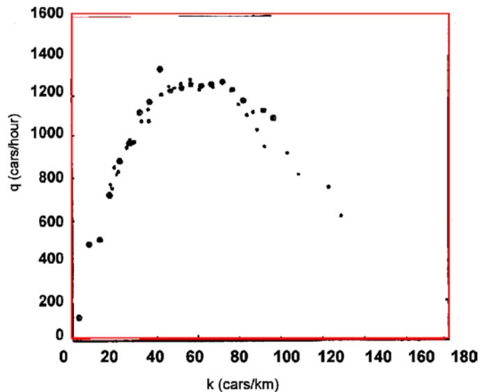
Note: The solid points are the flow values derived from the speed classes assuming steady-state condition. Also included in Figure 4.25 are one minute average flow values shown as encircled points.
