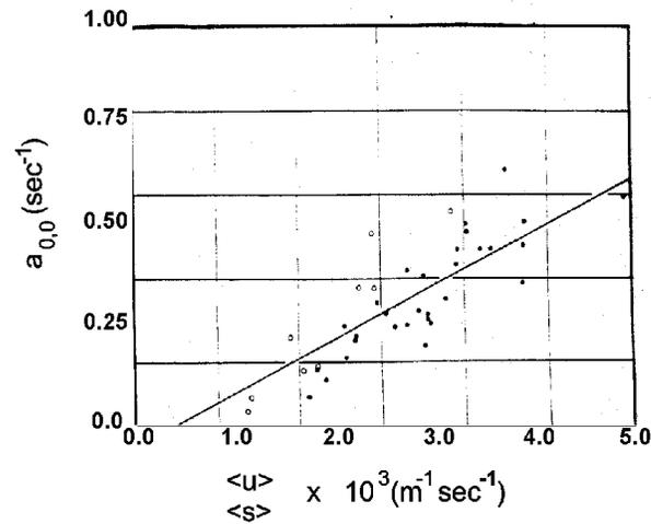
Note: The sensitivity coefficient versus the reciprocal of the average spacing for each bus following experiment. The least squares straight line is shown. The slope of this regression is an estimate of the reciprocal spacing sensitivity coefficient. The solid dots and circles are data points for two different test runs.
