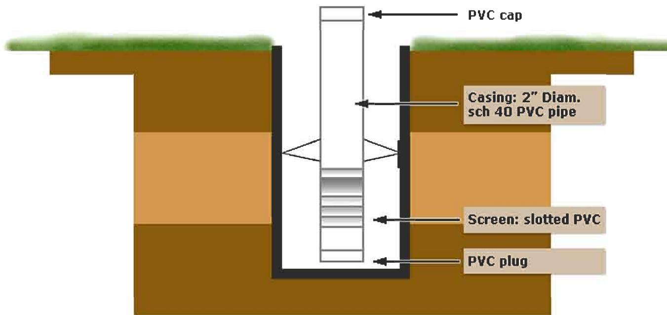
3. Install clean, coarse backfill to 1 ft height above top of screen
