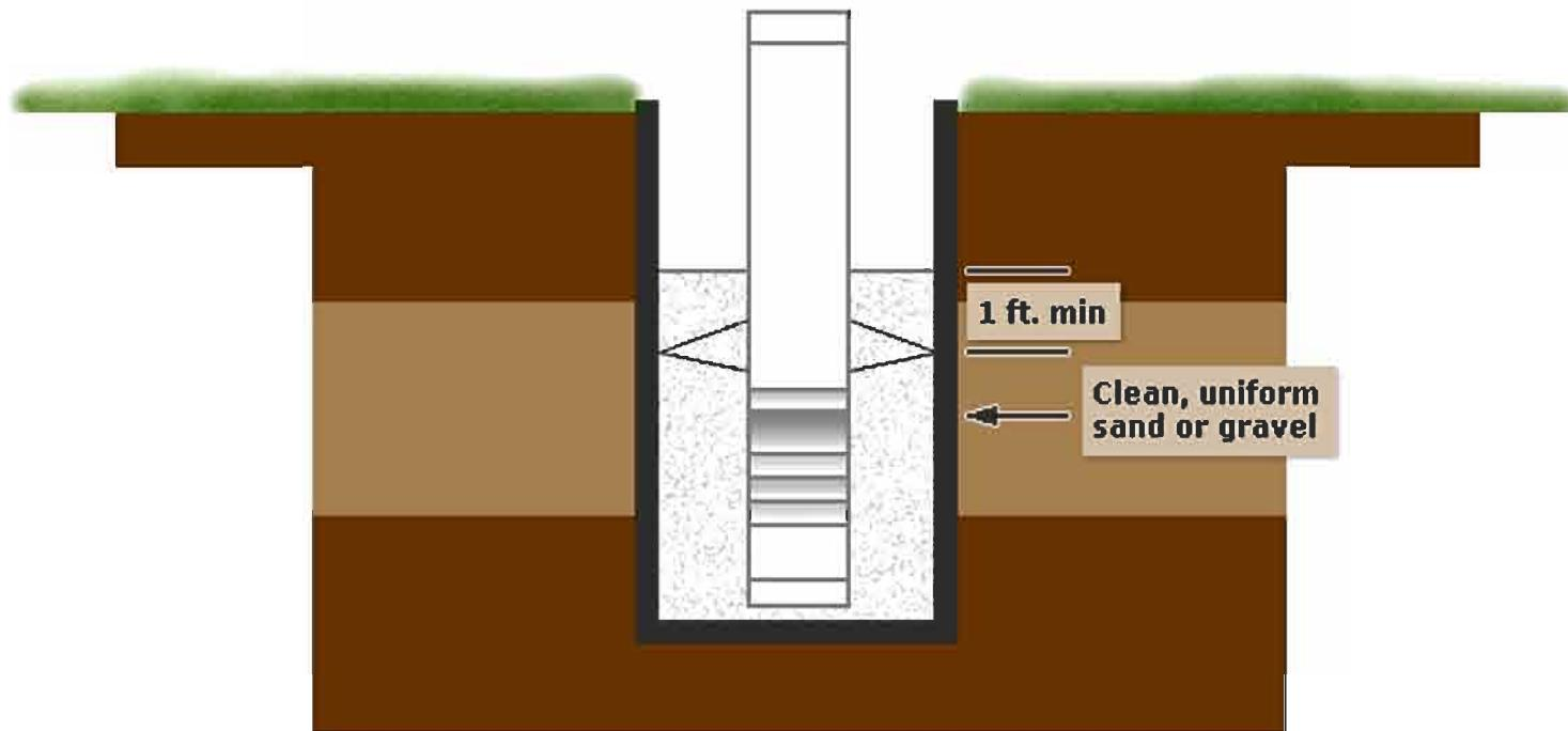
4. Add bentonite seal. Grout to surface pad. Wait 24 hr to develop.
