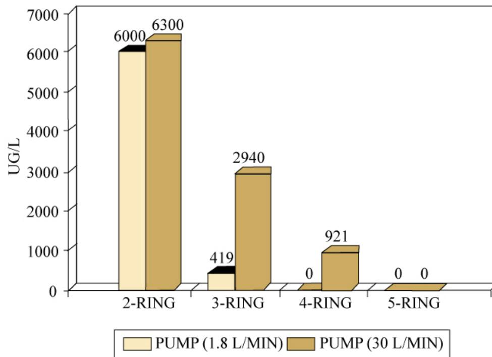
Source: MacFarlane, I. D., J. L. Kocornik, F. T. Barranco and A. R. Bonas (1992). The application of slow pumping at a manufactured gas plant. The Sixth National Outdoor Action Conference on Aquifer Restoration, Ground Water Monitoring and Geophysical Methods, Las Vegas, NV, Water Well Journal Publishing Company.
