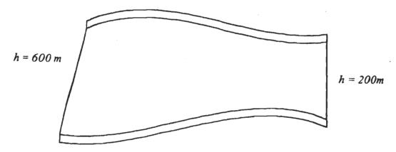
4. Draw a quantitatively accurate flow net for the case below. Show flow direction arrows on the flow lines. Calculate the volume discharge per meter thickness of section if  $K = 5 \times 10^{-2}$  cm/s (note the change in units for conductivity).
