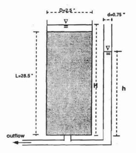
d) Use the data from the in-class demonstration (head in the manometer tube over time) to fit a value to the parameter K (hydraulic conductivity) in cm/sec. We are not necessarily looking for the best statistical fit, just a reasonable fit to the relation:
