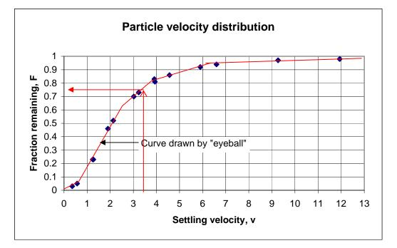
b.  $T_R = 2$  hours hydraulic residence time H = 4 m  $V_0 = \frac{4}{2} \frac{m}{hr} = 2 \frac{m}{hr}$  overflow rate  $= 3.3 \frac{cm}{min}$
