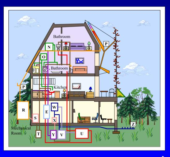
P—gutters R—rain water cistern S—combination filter T—drinkable cold water tank O—drinkable hot water tank
