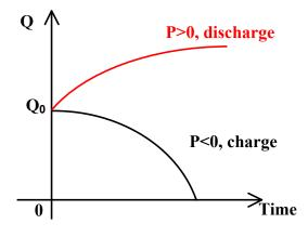
Figure 2: Q vs. time in constant power mode
