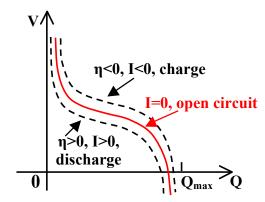
Figure 1: Typical "discharge curve" for a battery, showing the cell voltage versus state of charge at different currents.
