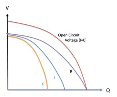
Fig 3. Battery discharge at constant power (P), constant current (I), and constant external resistance (R), compared to open circuit voltage versus state of charge.
