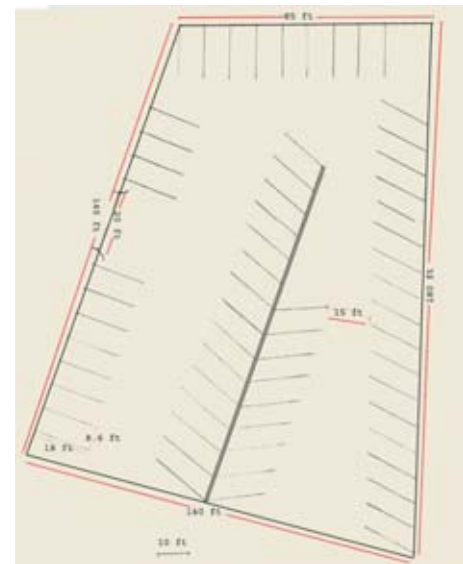
Figure 4.6b: Reconfiguration of Parking (40% capacity increase)
