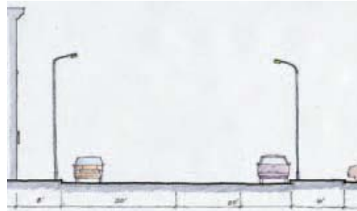
Figure 4: Existing section of Centre Street
