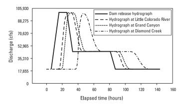
**Figure 13.** Hypothetical Glen Canyon Dam release and flow hydrographs designed to create a peak discharge of 100,000 cfs for 1 min at Diamond Creek, followed by a beach-building discharge of 45,000 cfs for a duration of 2 d.
