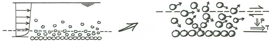
Figure 10-11. The “gravity-bed case”: a turbulent shear flow in a gravity field, transporting sediment particles denser than the fluid medium.
