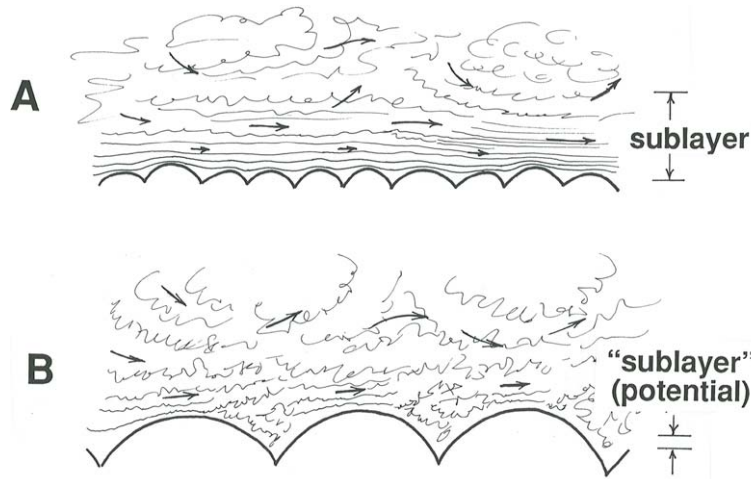
Figure 4-18. Differences in flow structure near a granular bed, depending upon whether A) the viscous sublayer is thicker than the heights of the particles or B) the heights of the particles are greater than what the thickness of the viscous sublayer would be in the absence of the particles.
