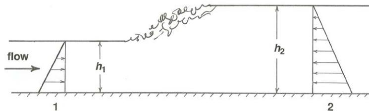
Figure 5-13. The hydraulic jump. The distribution of hydrostatic pressure is shown at section 1, upstream of the jump, and at section 2, downstream of the jump.
