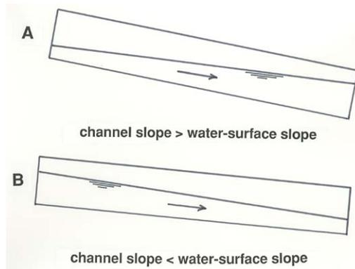
Figure 5-6. **A)** An open-channel flow for which the water-surface slope is less than the slope of the channel bottom. **B)** An open-channel flow for which the water-surface slope is greater than the slope of the channel bottom.
