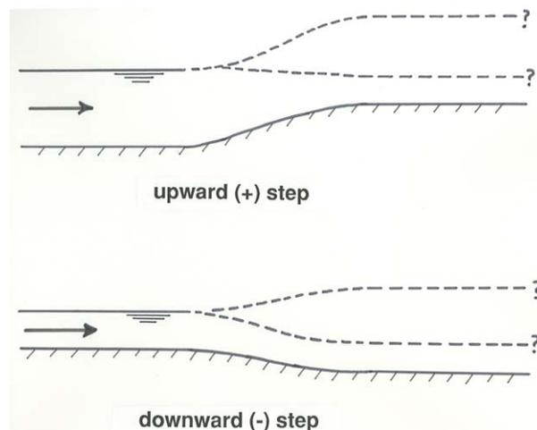
Figure 5-3. A positive step and a negative step in a channel bottom.
