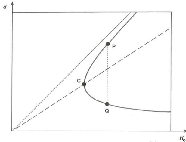
Figure 5-11. The specific-energy diagram for one particular value of  $q$ , to illustrate the effect of raising and then lowering the channel bottom to force the flow to pass from subcritical to supercritical.
