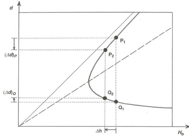
Figure 5-8. The specific-energy diagram for one particular value of  $q$ , to illustrate the effect of raising the channel bottom by a distance  $\Delta h$ . See text for explanation.
