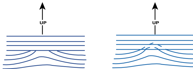
Figure 3-10. How contour lines represent overhangs.
