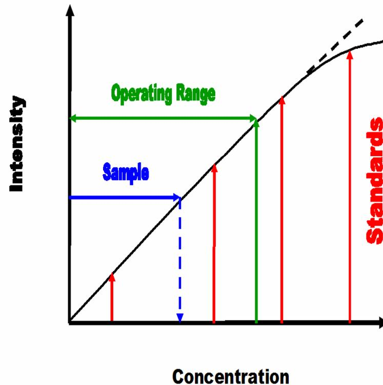
Figure 2. Calibration curve for quantitative analysis
