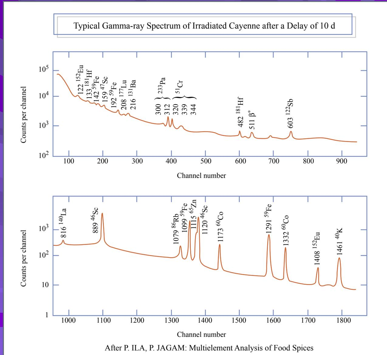
Figure 16. Multi-element gamma-ray spectrum of a food material
