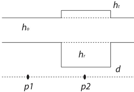
The figure shows the setup. If the mountain range is in isostatic equilibrium, the pressure at point 1 will equal the pressure at point 2. The additional mass of the mountain range of height  $h_t$  is compensated by the negative mass anomaly of the crustal root (thickness  $h_r$ ). To set up the equations, we equate the pressure at point 1 and point 2, and solve for the ratio  $h_t/h_r$ .
