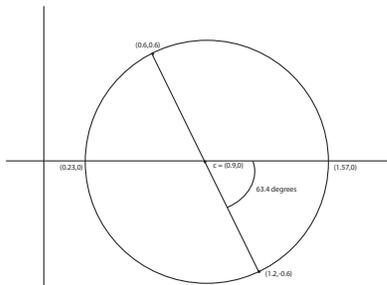
$\sigma_1 = 1.57\text{kbar}$ ,  $\sigma_3 = 0.23\text{kbar}$ . The angle between the normal to the first plane and  $\sigma_1$  is one-half of  $63.4^\circ$ , i.e.  $31.7^\circ$ . Note how the angle is measured.
