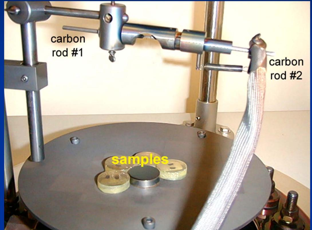
*To monitor coat-thickness, a polished brass block is coated with the samples*
