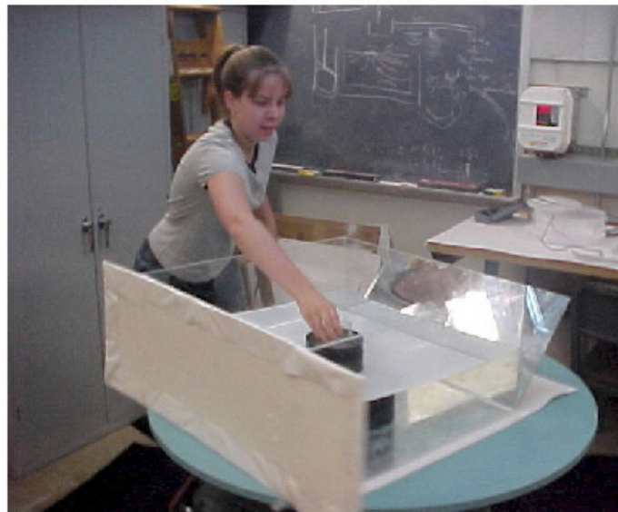
Figure 3: The cylinder collapse experiment.
