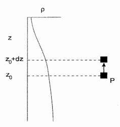
Figure 3.9: Displacement of a water parcel P in stable stratification.
