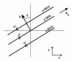
Figure 3.10: Phase lines and motions within a plane internal gravity wave.
