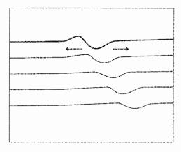
Figure 3.2: Interfacial (internal) waves in a fluid with many constant-density layers.
