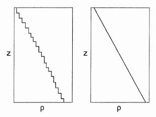
Figure 3.3: Density stratification of a fluid with (left) density steps and (right) continuous stratification.
