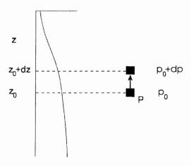
Figure 3.6: Vertical displacement of a compressible air parcel.
