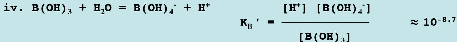
These “apparent constants” are functions of temperature, salinity, and pressure.
