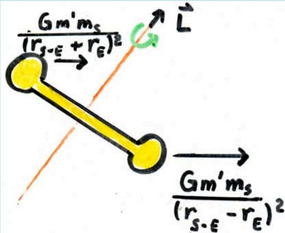
Precession frequency depends on angular momentum and torque
